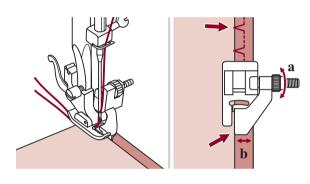
Place the fabric under the foot. Turn the handwheel forwards by hand until the needle swings fully to the left. It should just pierce the fold of the fabric. If it does not, adjust the stitch width accordingly.
