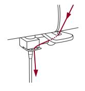
7. Pass the thread behind the flat, horizontal thread guide.
