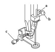
Remove the presser foot holder, and attach the darning foot to the presser foot holder bar.
