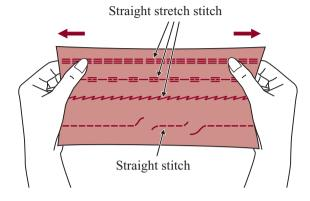
It assures you of a stitch that is strong and flexible and will give with the fabric without breaking. Good for easy to ravel and knit fabrics. It is good for joining durable fabric such as denims.
