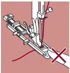
Position the fabric so that the needle is 2mm (1/16 inch) in front of the area to be darned, and then lower the presser foot lever.
