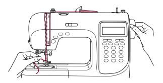
1. Hold the upper thread with the left hand. Turn the handwheel towards you (counterclockwise) lowering, then raising the needle.
