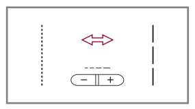
To shorten the stitch length, press the "-" button (left). For a longer stitch length, press the "+" button (right).
