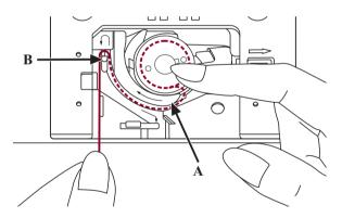
With a finger held gently on top of the bobbin. Draw the thread at the arrow markings into the stitch plate thread guide from (A) to (B).
