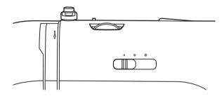
The speed limiting adjustment lever can control the sewing speed. To increases the speed, slide the lever to the right, to decrease the sewing speed, slide the lever to the left.
