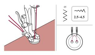
Select zig zag pattern. Adjust the stitch width to "2.5-4.5" according to the distance between the two holes of the button.
