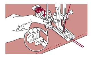
Pull the buttonhole lever all the way down and position it behind the bracket on the buttonhole foot.
