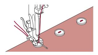
Before sewing, press the Auto-lock button to sew reinforcement stitches automatically at the beginning and at the end of the stitch.
