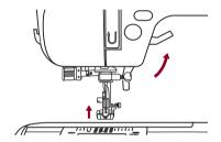
Lift the presser foot lifter to raise the presser foot bar.
