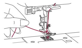
2. Gently pull on the upper thread to bring the bobbin thread up through the needle plate hole. The bobbin thread will come up in a loop.
