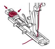
Attach the buttonhole foot, then pull out the button holder plate and insert the button.
