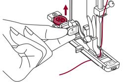
Buttonholes are sewn from the front of the presser foot to the back, as shown.
