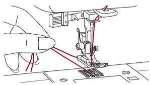
3. Pull both threads to the back under the presser foot
