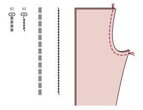
Straight stretch stitch is used to add triple reinforcement to stretch and hardwearing seams.
