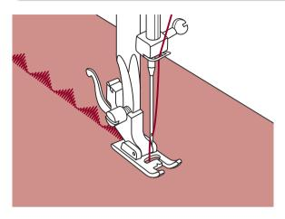
Use the satin stitch foot for satin stitching and sewing decorative stitches. This foot has a full indentation on the underside to allowed easy sewing over the thickness of the stitches form by closely spaced zigzag stitches, and even feeding of the fabric.
