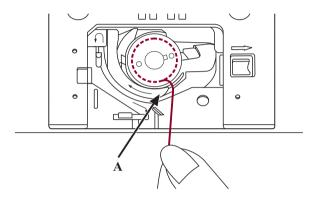
Pull the thread through the slit (A).
