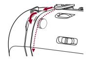
4. Thread the tension module by passing the thread between the silver discs.
