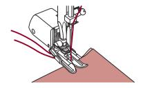
Draw the bobbin thread up and place both the bobbin thread and the needle thread behind the walking foot attachment.
