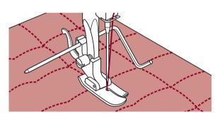
Sew the first row and move over the fabric to sew successive rows with the guide riding along the previous row of stitching.
