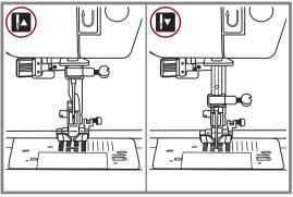
Press the button so that the arrow, on the LCD screen, will point upward " \[ \] " and the needle will stop in the highest position. When you press the button so that the arrow points downward " , the machine will stop with the needle in the lowest position.
