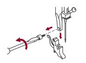
Remove the presser foot holder by unscrewing (counterclockwise) the presser bar attaching screw.
