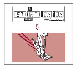
Press foot controller. The machine will start to sew from first entered pattern. On the LCD screen, sewing stitch data is indicated.
