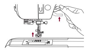
When sewing several layers or thick fabrics, the presser foot can be raised a second stage for easy positioning of the work.
