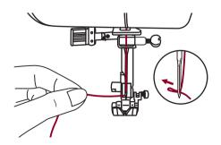
Hold the thread loosely and release the lever slowly. The hook will turn and pass the thread through the needle eye forming a loop.
