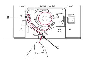
Pull the thread at the arrow markings into the stitch plate thread guide from (B) to (C).
