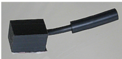
Magnet Arm for Lace Carriage
